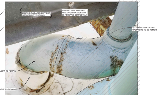
⑤ DETAIL - PIPE PENETRATION DOWN THRU ROOF - DEMOLITION SCALE: NONE
