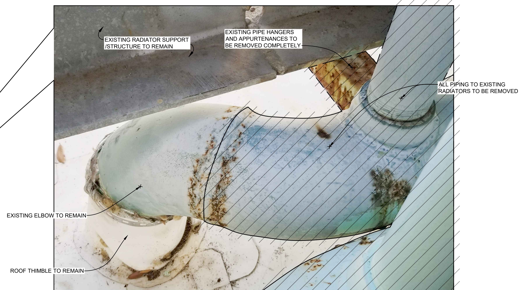
B DETAIL - PIPE PENETRATION DOWN THRU ROOF - DEMOLITION SCALE: NONE
