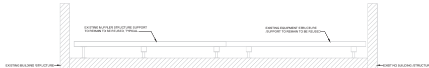
2 SECTION - ROOF EQUIPMENT STRUCTURE - DEMOLITION SCALE: NONE
